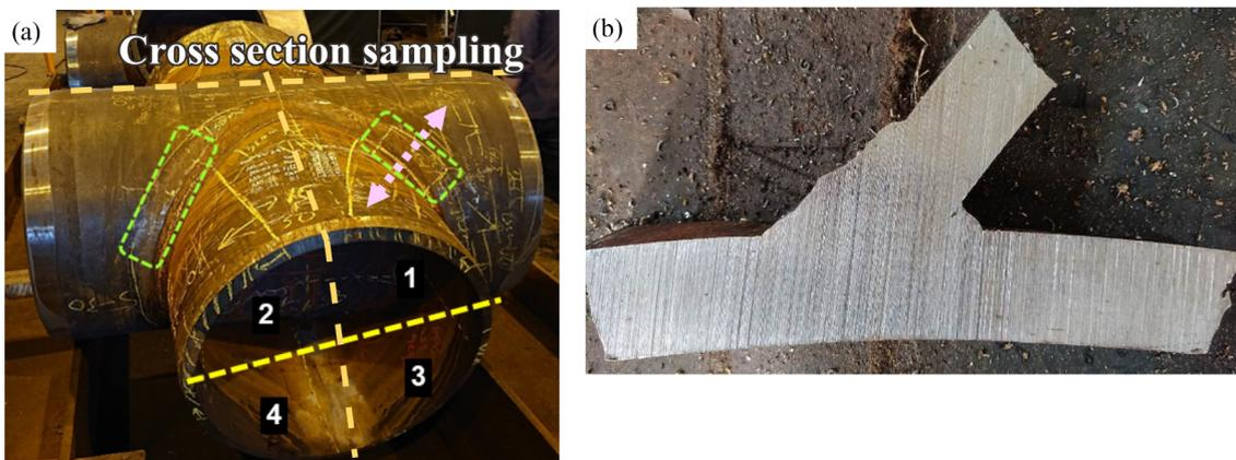
**Fig.4.** Sampling preparation of the welded node. (a) cutting indications, (b) cross-section of the weld.
