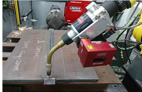
**Fig.5.** Lincoln S-500, combined with a Fanuc M20iA robot, performs welding in the laboratory.
