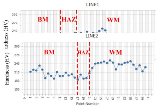
Fig.10. Hardness distribution of welding cross-section of a node.
